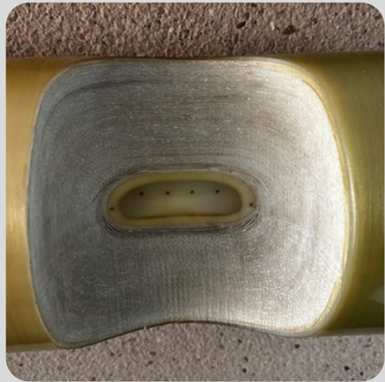
Cutaway showing the spiral-wound membrane sheets and central permeate tube within the fiberglass pressure shell.
