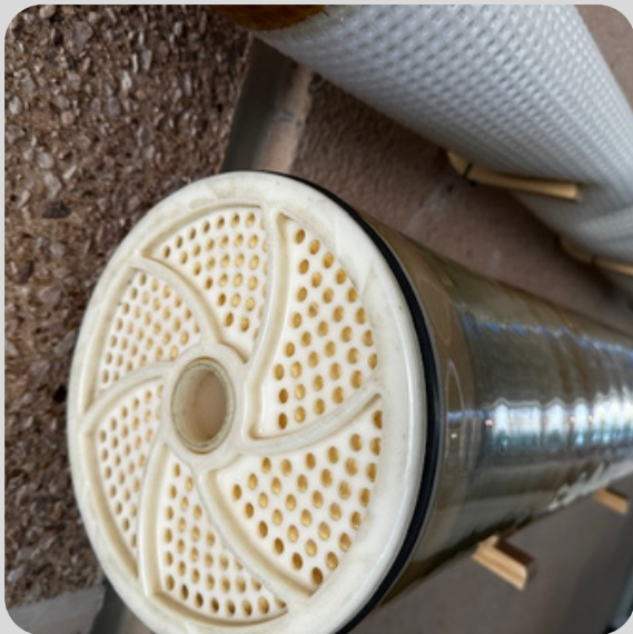
End cap view showing the feed water inlet, radial flow channels, and O-ring seal of an intact RO membrane module
