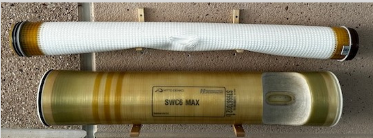
RO Membrane from SA Desalination Plant Top: Exposed internal structure showing permeate tube and membrane layers; Bottom: Intact Hydranautics SWC6 MAX RO membrane with outer fiberglass casing.
